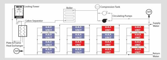
Consider a two-pipe closed loop water circuit, through which non-refrigerated water is circulated continuously throughout the building. In moderate weather, units serving the shady side of a building are often heating, while those serving the summer are cooling. When approximately one third of the units in operation are cooling, they add sufficient heat to the water loop so that it is not required to add or remove heat from the water loop.
